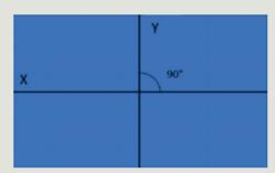
Setting this axis up is crucial and it's good practice to check all angles and measurements are correct at this stage before any planks are laid.
